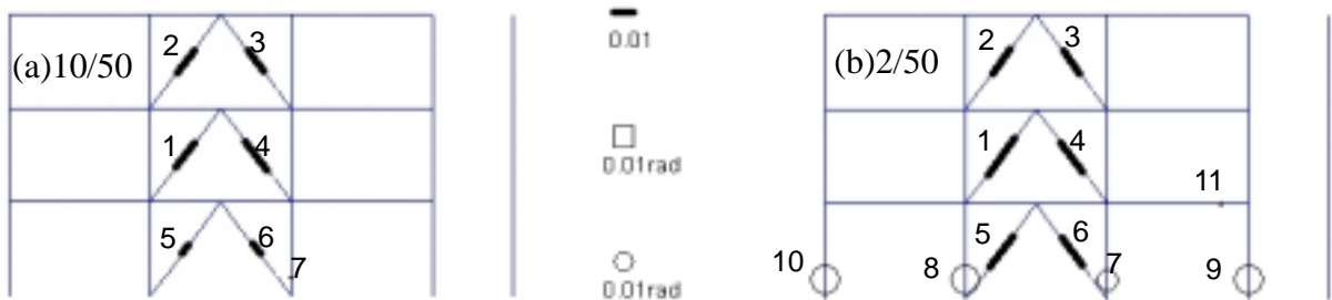
Fig. 25 Plastic hinge distributions obtained from VISA2D program
